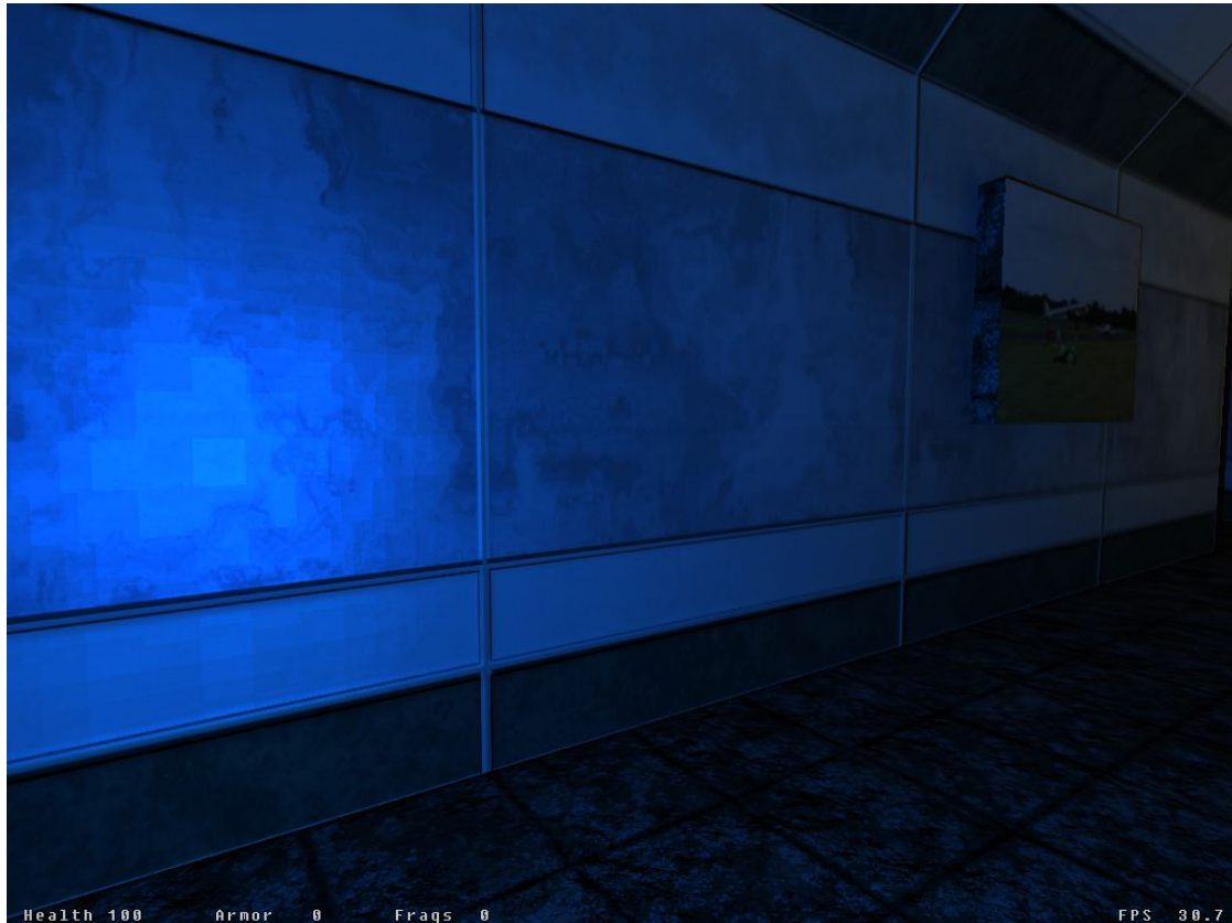
Figure 29: A blocky specular highlight on an NVidia NV2X GPU.
